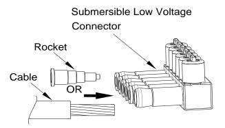
Insert the cable into the tower (250 to 350 kcmil) or the rocket (#12 to 4/0) until the end of the conductor reach the end of the window.
