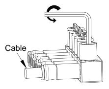
Insert torque tool and rotate it.(120in-lb for #12 to #4, 240in-lb for #2 to 350kcmil)
