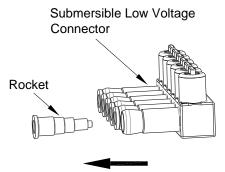
Remove the rocket (the rocket is not required for 300/350 kcmil).
